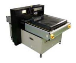
X-Y Stage machining for glass mask
